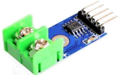
SEN19A 8.320 MAX6675, Sensor de Temperatura 0 a 800° - MAX6675
