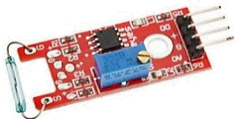
M022 4.480 Modulo Reed Switch, Interruptor electromagnetico 5v
