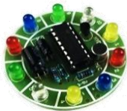
M050B 7.600 Lampara led giratoria, control de voz kit cd4017
