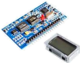
MO82 32.640 Inversor onda sinusoidal pura EG8010+IR2110 Pantalla y modulo
