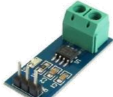
SEN13-30 30amp 4.352 ACS712, sensor de corriente AC/DC - 30amp
