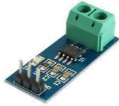
SEN13-20 20amp 6.800 ACS712, sensor de corriente AC/DC - 20amp
