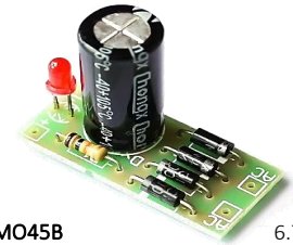
MO45B 6.720 1N4007 Conversor de Corriente AC a DC - 12v
